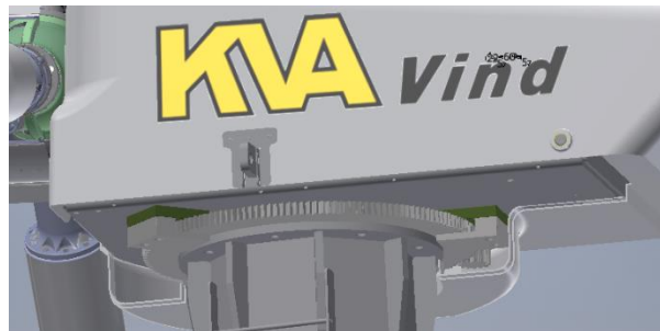
Figure 4. The view for installation of yaw system on KVA Wind 10-15
